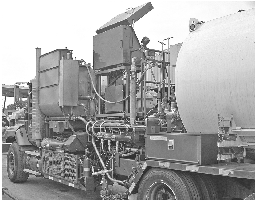
Figure 37 - Truck Mounted Triplex Pump
