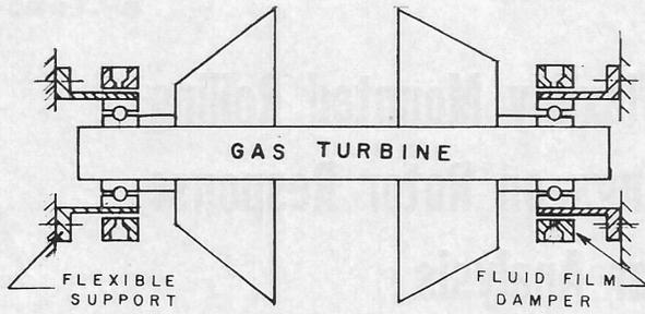
Fig. 1 Schematic diagram of the general rigid body rotor
