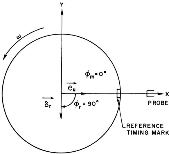
Fig. 17 Rotor schematic for sample balance problem
