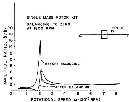
Fig. 20 Experimental response curves before and after balancing to zero at 2050 rpm
