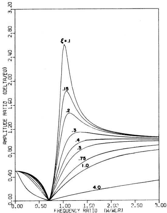
Fig. 6 Response curves with  $\bar{\delta}_r = 0.5$ ,  $\phi_r = 180$  deg for various damping ratios
