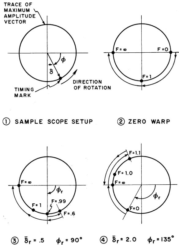
Fig. 16 Schematic showing the movement of the timing mark on an oscilloscope screen as speed increases for various  $\bar{\delta}_r$  and  $\phi_r$  values (for damping ratios below critical damping)
