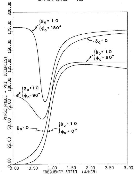
Fig. 24 Phase angle curves with zero residual bow and various values of mechanical runout
