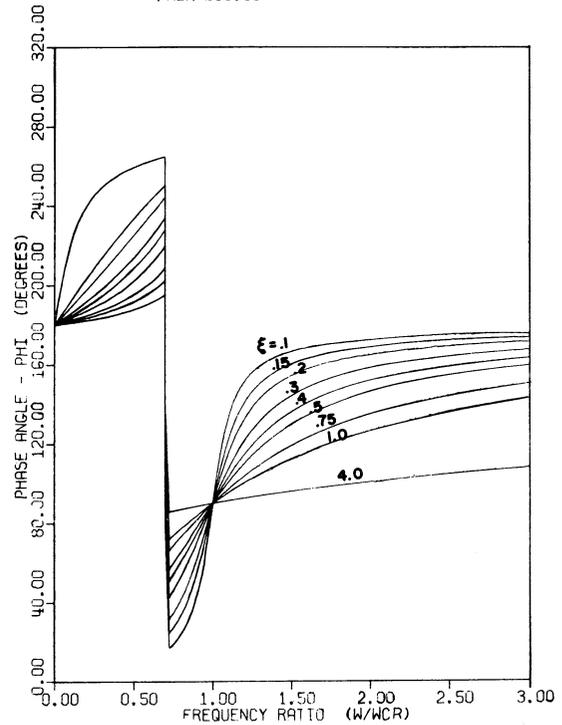
Fig. 7 Phase angle curves with  $\bar{\delta}_r = 0.5$ ,  $\phi_r = 180$  deg for various damping ratios
