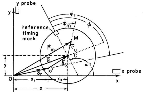
Fig. 1 Single mass flexible rotor with bowed shaft, end and side views
