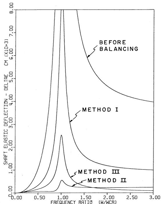
Fig. 22 Elastic response curves before and after balancing a bowed shaft by balancing Methods I, II, and III
