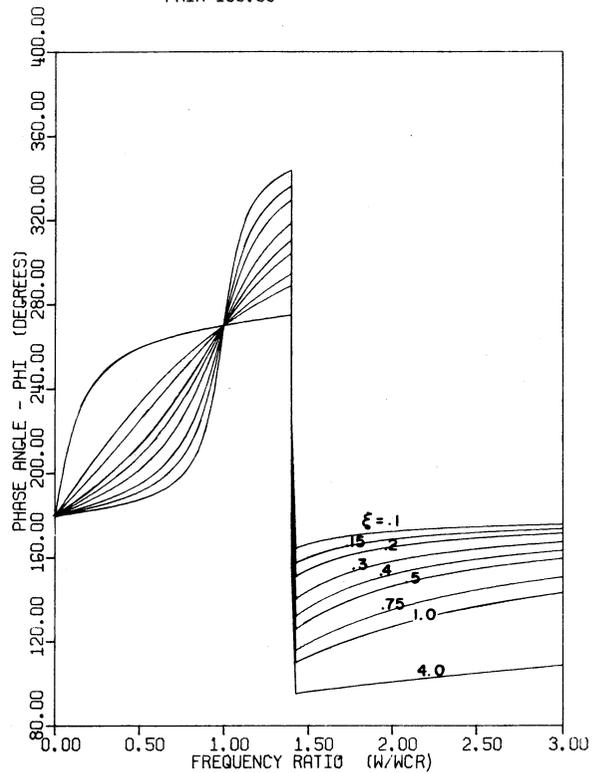
Fig. 12 Phase angle curves with  $\bar{\delta}_r = 2.0$ ,  $\phi_r = 180$  deg for various damping ratios
