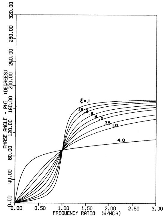
Fig. 3 Phase angle curves with zero residual warp for various damping ratios
