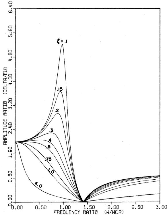
Fig. 11 Response curves with  $\bar{\delta}_r = 2.0$ ,  $\phi_r = 180$  deg for various damping ratios
