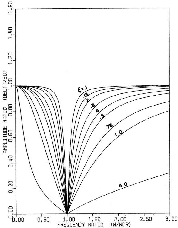
Fig. 15 Response curves with  $\bar{\delta}_r = 1.0$ ,  $\phi_r = 180$  deg for various damping ratios, balanced rotor (out of phase response)
