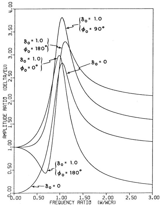
Fig. 23 Response curves with zero residual bow and various values of mechanical runout
