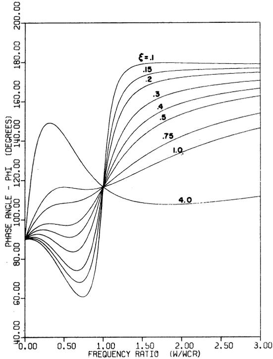
Fig. 5 Phase angle curves with  $\bar{\delta}_r = 0.5$ ,  $\phi_r = 90$  deg for various damping ratios
