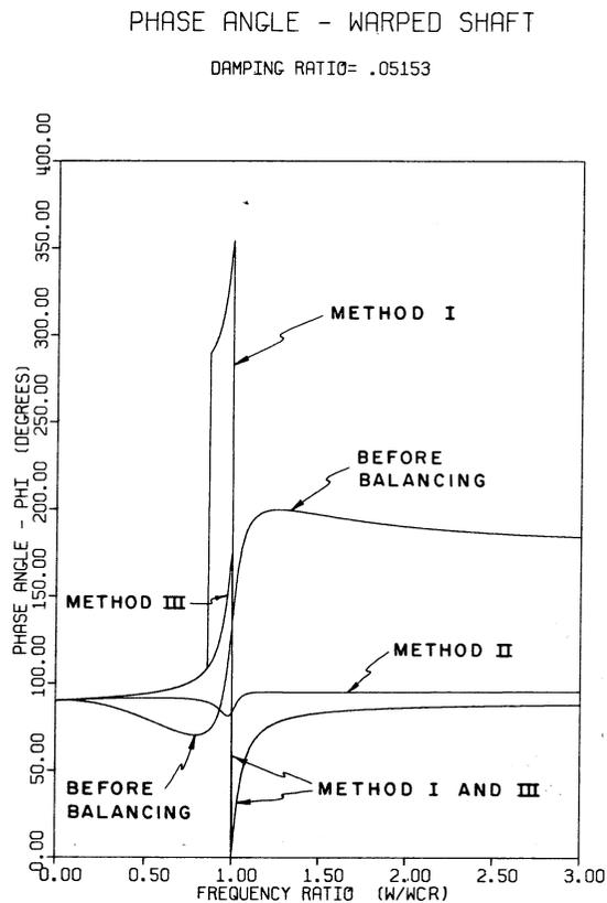
Fig. 19 Phase angle curves before and after balancing a bowed shaft by balancing Methods I, II, and III
