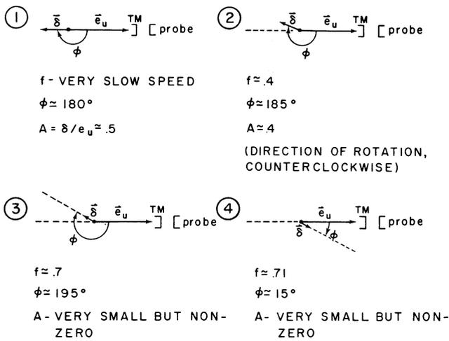
Fig. 8 Vector diagrams showing the 180 deg phase shift at  $f = 0.7071$  for  $\bar{\delta}_r = 0.5$ ,  $\phi_r = 180$  deg
