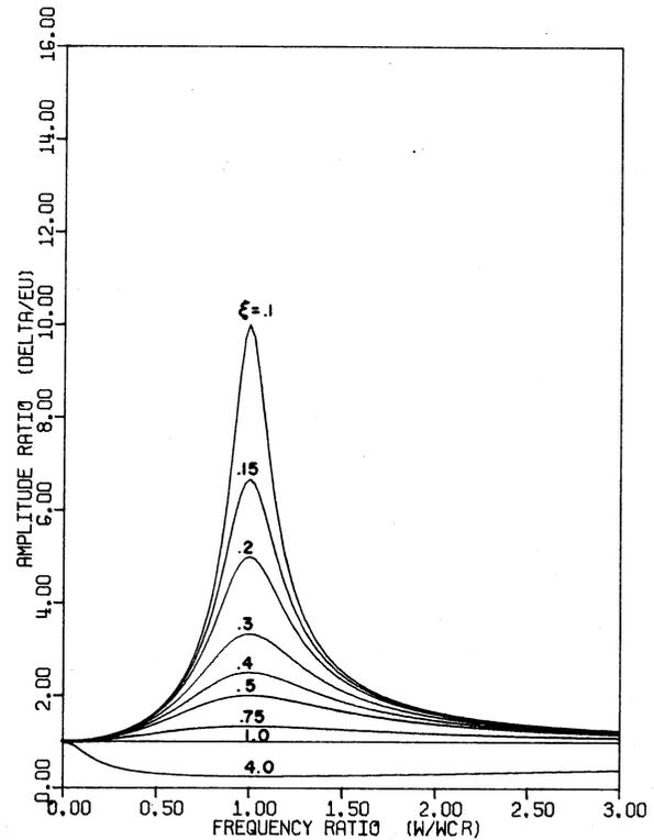
Fig. 14 Response curves with  $\bar{\delta}_r = 1.0$ ,  $\phi_r = 0$  deg for various damping ratios (in-phase response)
