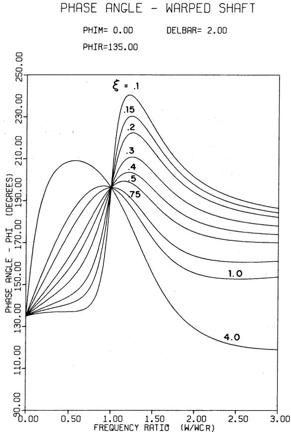
Fig. 13 Phase angle curves with  $\bar{\delta}_r = 2.0$ ,  $\phi_r = 135$  deg for various damping ratios
