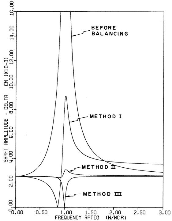
Fig. 18 Response curves before and after balancing a bowed shaft by balancing Methods I, II, and III
