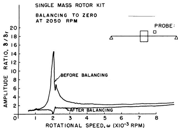
Fig. 21 Experimental response curves before and after balancing to zero at 1800 rpm
