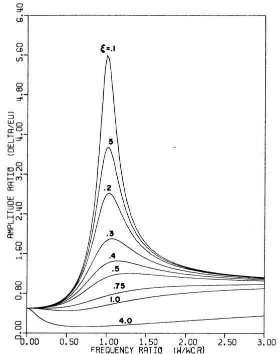
Fig. 4 Response curves with  $\delta_r = 0.5$ ,  $\phi_r = 90$  deg for various damping ratios
