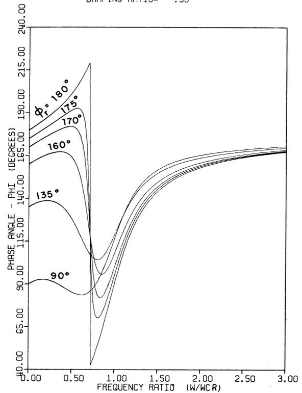
Fig. 10 Phase angle curves with  $\bar{\delta}_r = 0.5$ ,  $\xi = 0.3$  for various  $\phi_r$  values
