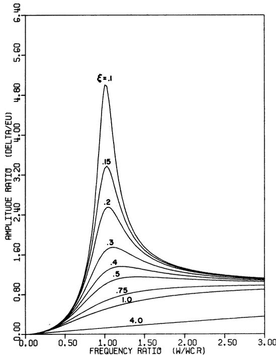
Fig. 2 Response curves with zero residual warp for various damping ratios
