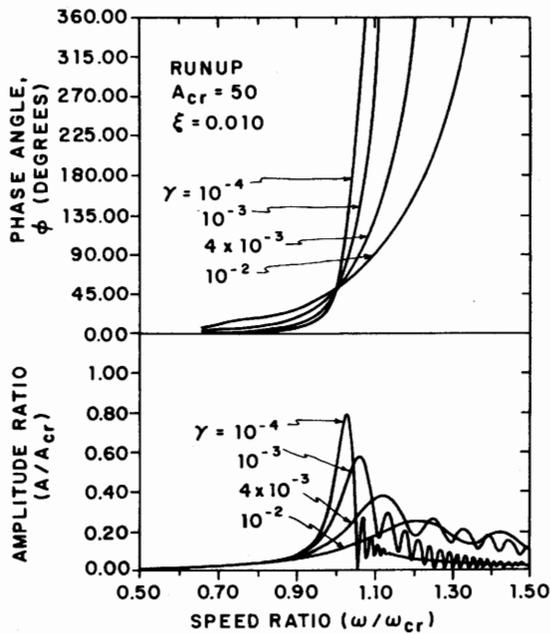
Fig. 2 Critical speed response for runup for  $\zeta = 0.010$
