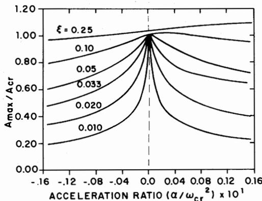
Fig. 8 Summary of maximum amplitude dependence on acceleration rate and damping
