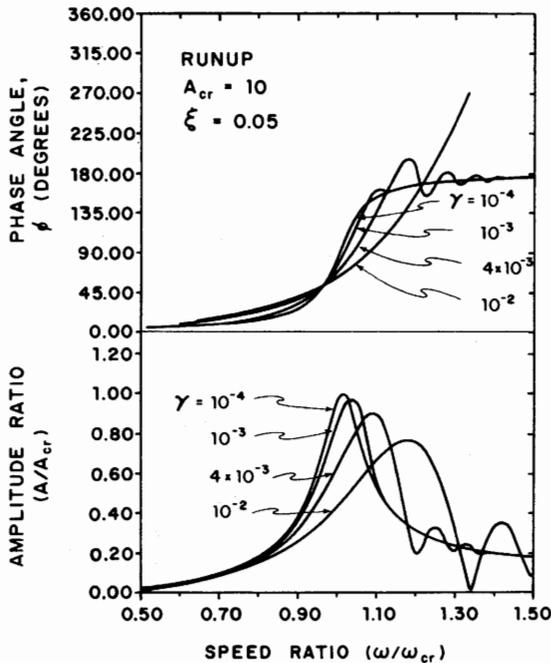
Fig. 4 Critical speed response for runup for  $\zeta = 0.05$
