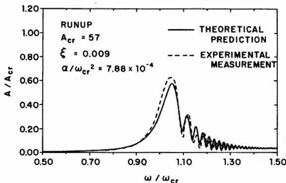
Fig. 11 Typical experimental critical speed response and theoretical predictions
