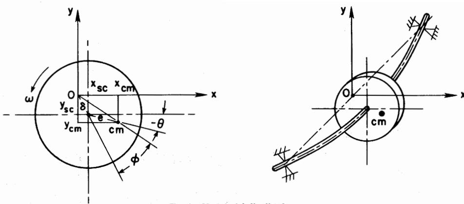
Fig. 1 Model of Jeffcott rotor
