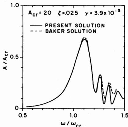
Fig. 7 Comparison of present and Baker [2] critical speed response predictions for runup for  $\zeta = 0.025$
