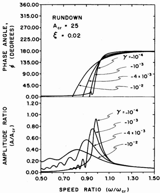
Fig. 6 Critical speed response for rundown for  $\zeta = 0.02$
