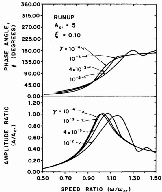
Fig. 5 Critical speed response for runup for  $\zeta = 0.10$
