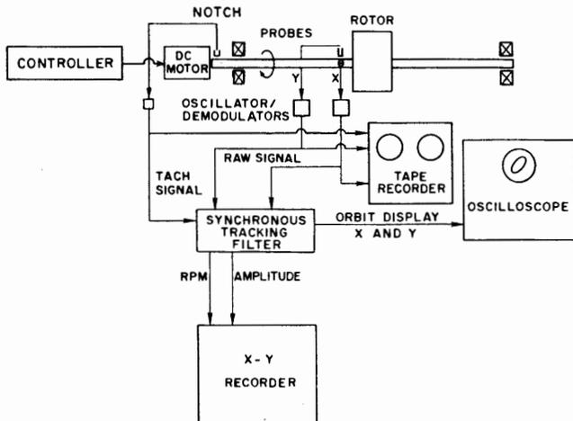
Fig. 10 Test rotor and instrumentation
