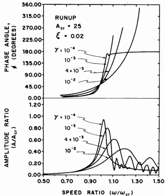
Fig. 3 Critical speed response for runup for  $\zeta = 0.02$
