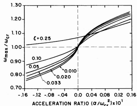
Fig. 9 Critical speed shift as a function of acceleration rate and damping
