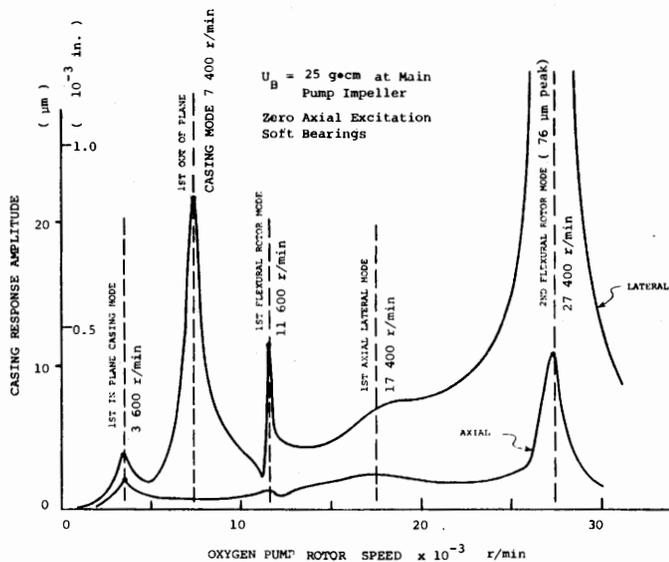
**Fig. 7 Lateral and axial steady-state response amplitudes at casing preburner pump end due to main pump impeller unbalance**
