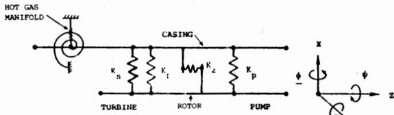
**Fig. 6 Space Shuttle Main Engine oxygen pump computer simulation lumped parameter model ( $K_p$  - pump bearing,  $K_z$  - balance piston,  $K_t$  - turbine bearing,  $K_s$  - turbine seals)**
