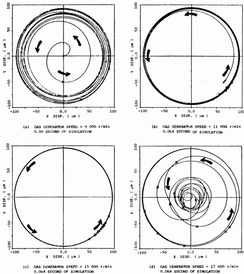
**Fig. 4 Nonlinear transient rotor orbits at squeeze film damper bearing showing nonlinear jump (→ direction of rotor precession)**
