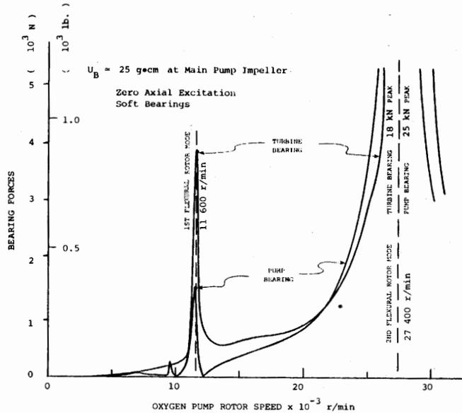
**Fig. 8 Bearing forces in the  $x$ -direction due to main pump impeller unbalance**
