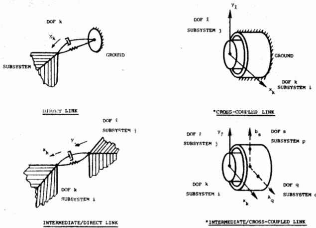
Fig. 1 Linearly elastic connection types in component mode synthesis (\* Figures show  $l=j$  and  $o=p$ )
