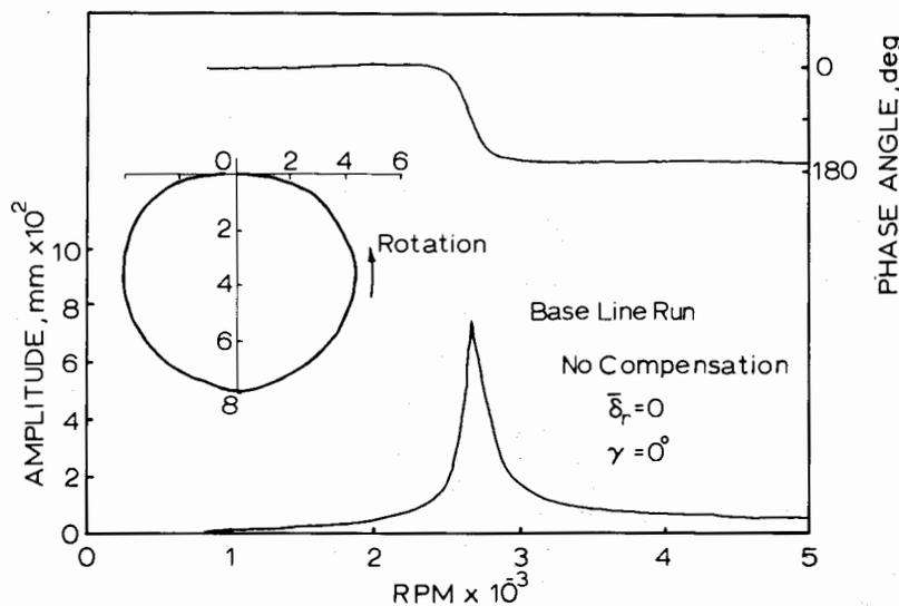
Fig. 11 Base line response ( $\delta_r = 0, \gamma = 0$  deg)
