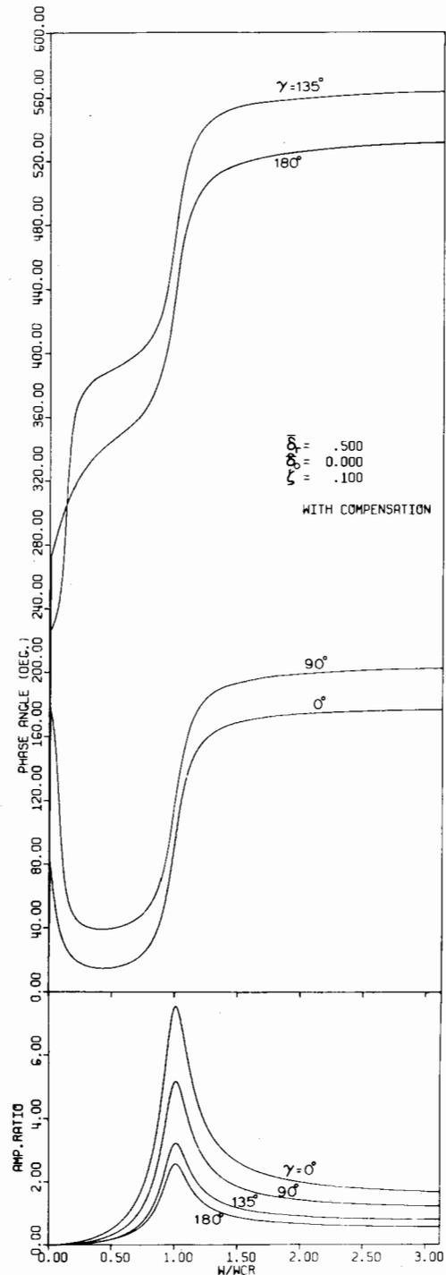
Fig. 8 Response curves with compensation for  $\zeta = 0.1$  and  $\delta_r = 0.5$  for various  $\gamma$  values
