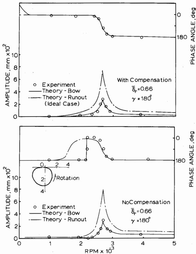
Fig. 14 Response curves for  $\delta_r = 0.66$  and  $\gamma = 180$  deg
