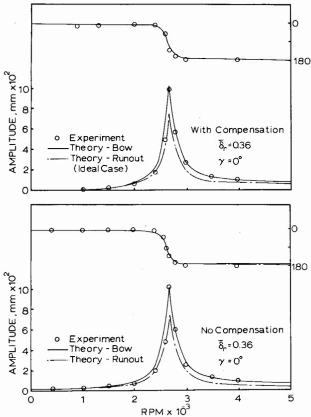
Fig. 12 Response curves for  $\delta_r = 0.36$  and  $\gamma = 0$  deg
