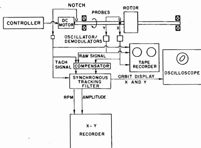
Fig. 10 Instrumentation used
