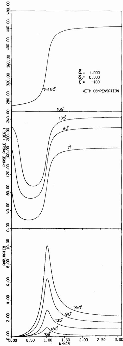
Fig. 4 Response curves with compensation for  $\zeta = 0.1$  and  $\delta_r = 1.00$  for various  $\gamma$  values
