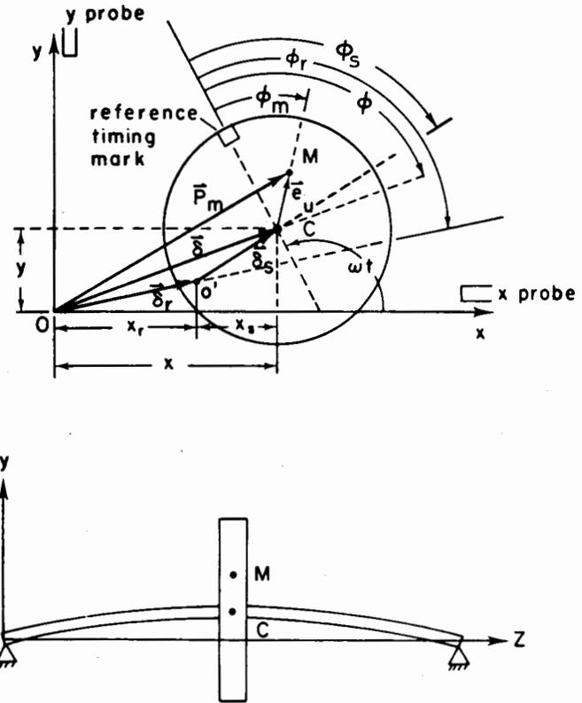
Fig. 1 Single mass flexible rotor with bowed shaft, end and side views
