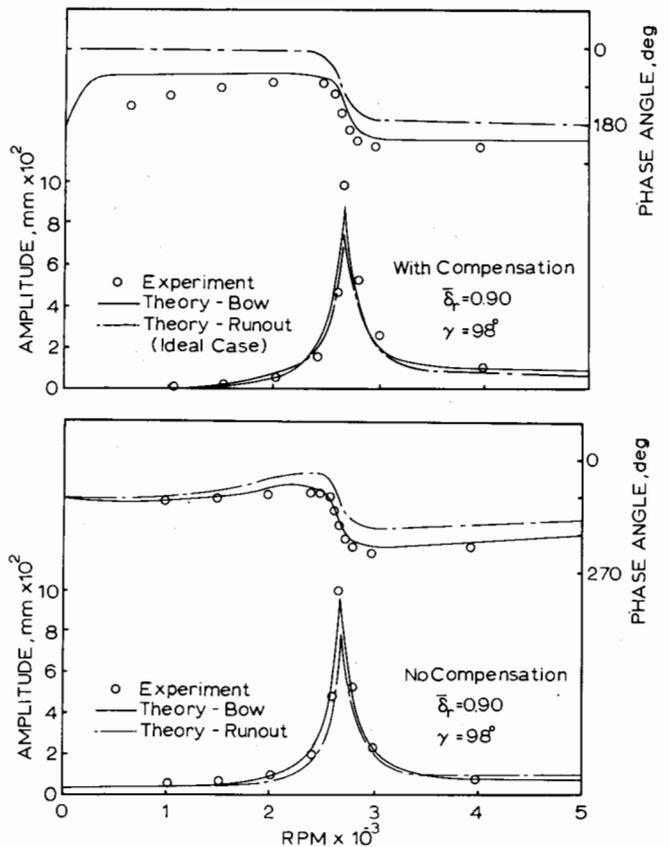
Fig. 13 Response curves for  $\delta_r = 0.90$  and  $\gamma = 98$  deg
