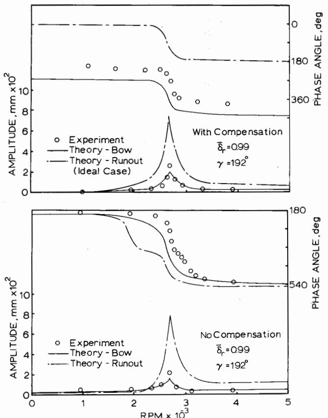
Fig. 15 Response curves for  $\delta_r = 0.99$  and  $\gamma = 192$  deg
