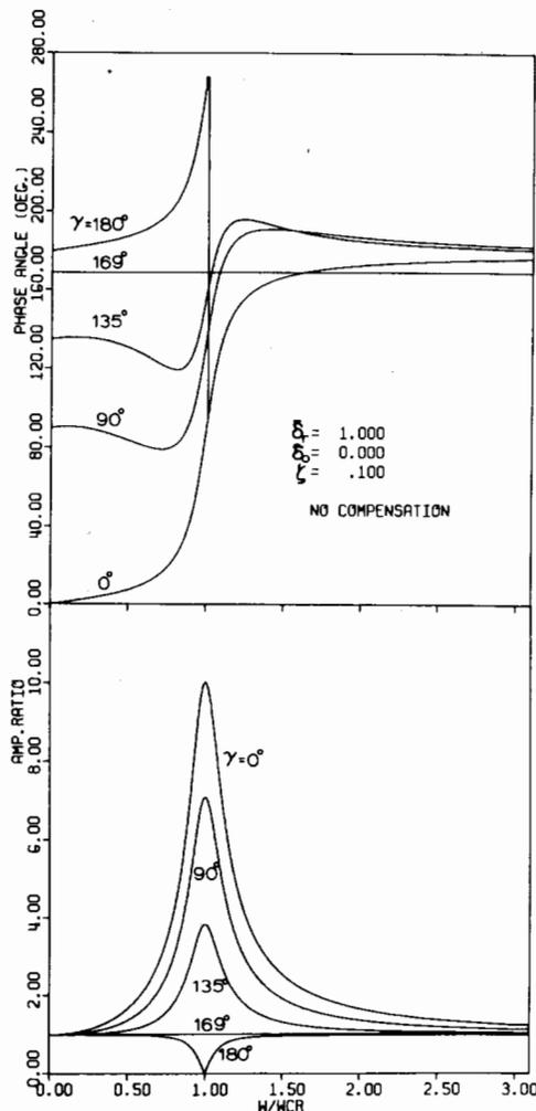
Fig. 2 Response curve without compensation with  $\zeta = 0.1$  and  $\delta_r = 1.00$  for various  $\gamma$  values
